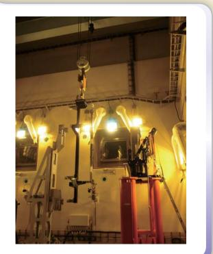
adjust the length of the hanging wire or rope in order to keep the balance. Also, the "Muon Attachment" must have two hanging positions with a precise alignment, because it has two weight centers, one with the "Muon Target" and another without. Furthermore, because a manual guidance against the swing or the rotation of the "Muon Attachment" is impossible, a definitive and careful crane operation is required. The precise position of the crane can be known outside through an encoder device.
