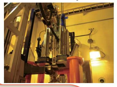
backward motion, and rotation. Then a rod, onto which the "Muon Target" is fixed, is held by the "Muon Attachment". Four fixing screws are loosened by a power-manipulator, which has a function of handling the screws for remote handling. It is difficult to know the precise position of the "Muon Attachment" from the outside of the "Hot Cell". Therefore, the loads of each motion are measured to monitor any unusual circumstances such as sticking out of an alignment pin and so on.
