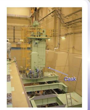
MLF building. For transportation, the "Muon Target" is remotely and automatically brought into a shielding vessel, which is called the "Muon Transfer Cask". In the "Hot cell", the used "Muon Target" is replaced with a new "Muon Target" through remote handling apparatuses. The used "Muon Target" is cut into pieces, thrown away into a dedicated storage container and kept under control.
