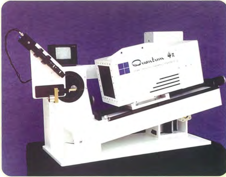
Figure 1. CCD automatic data collection system.
