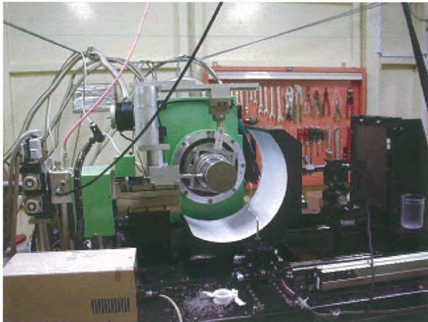
BL-1B MPD system reconstructed for single-crystal analysis at low temperature
