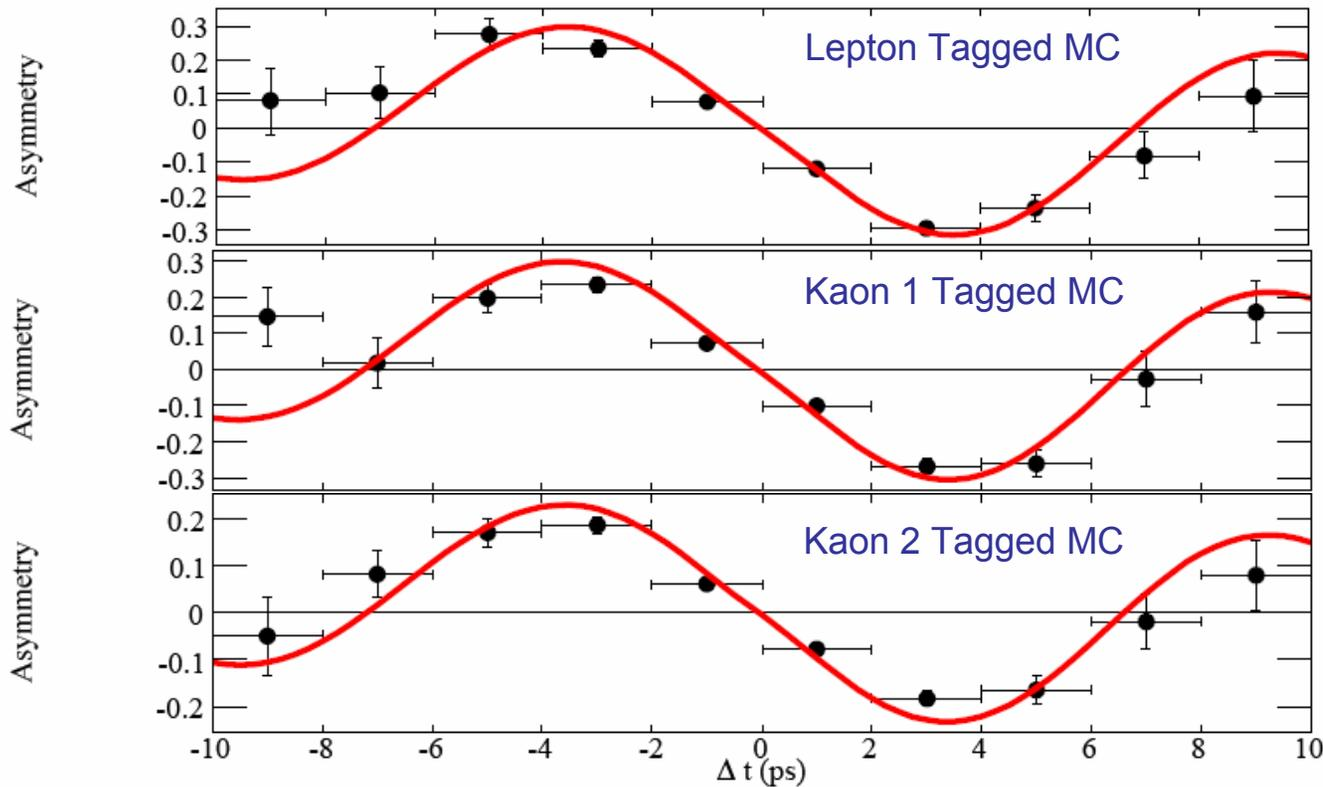
Amplitude of oscillation decreases for a given S and C as the mistag probability  $\omega_c$  increases.
