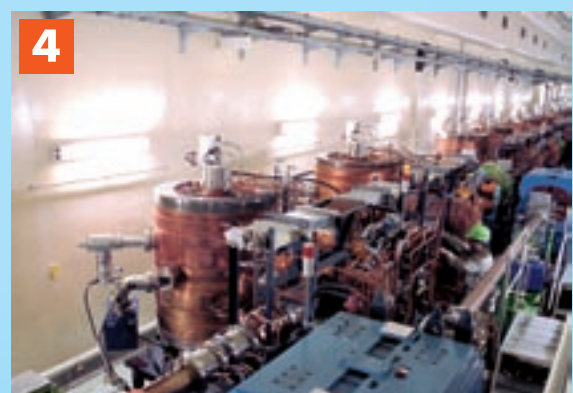
Normal-conducting radio-frequency cavity (ARES): The ARES cavities provide energy to the beams by accelerating them with the electromagnetic waves. The three-cavity combination is a unique design developed specifically for the purpose of handling high beam currents.
