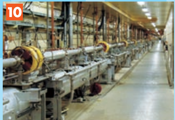
Injector: The powerful linear accelerator provides KEKB's double rings with 8 billion electron-Volt electron beams and 3.5 billion electron-Volt positron beams. The injector is a multi-purpose accelerator, also feeding beams to other electron accelerators located at KEK.
