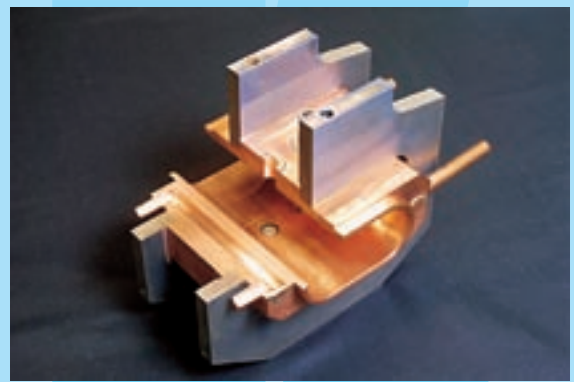
A beam position monitor block: A button-shaped electrode monitors the beam position by detecting the electrical signals from the beam. The monitor blocks are integrated into the beam ducts. Each ring employs more than 400 beam position monitor blocks.
