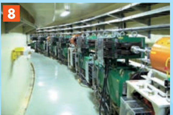
Beam transport line: Beams are delivered from the injector to the storage ring by the beam transport line. The delivery line consists of upper and lower lines for delivering positron and electron beams, respectively.
