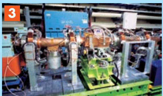
Steerable mask: Masks installed inside beam ducts prevent off-trajectory particles from hitting the detector, reducing the detector noise. The ducts themselves are movable, allowing control over the distance between beam and mask. They are installed in various locations in the rings.
