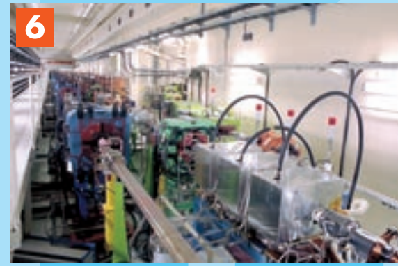
Injection point: This is the entry point of the beams delivered from the injector into the storage ring. An electromagnet installed at this point pulses the magnetic field inside at high frequency in order to efficiently feed new beams into the circulating beams in the storage ring.
