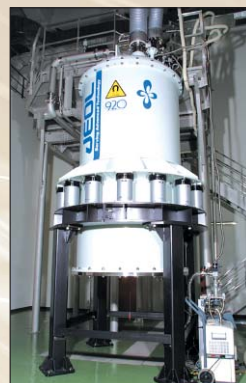
920-MHz NMR facility providing highest resolution in the world.
