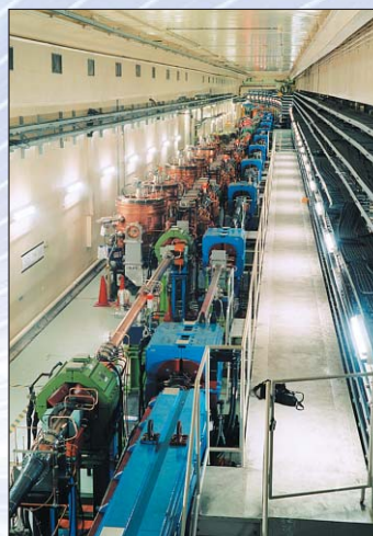
The world-highest beam intensity electron-positron collider, "B factory," generates massive amounts of B meson and anti-B meson pairs.
