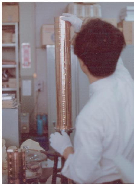
Figure 6: Stacking OFC disks and cylinders
