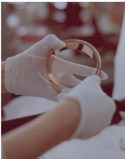
Figure 5: Fitting a silver alloy brazing wire into a groove on an OFC cylinder
