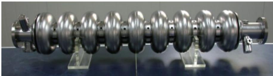
Peking University has a lot of experiences on the manufacturing of 9-cell TESLA-type cavities.
