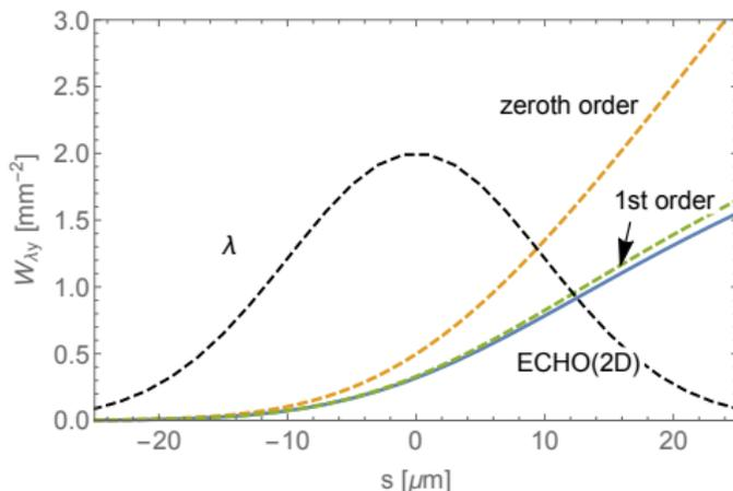
*Example calculation for LCLS dechirper:  $a = 0.7$  mm,  $y = 0.5$  mm. The above analytical result is given by green dashes, numerical ECHO(2D) results by the blue curve. The Gaussian bunch shape ( $\sigma_z = 10$   $\mu\text{m}$ ), with head to the left, is given in black dashes*
