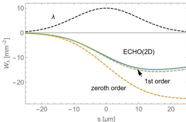
*Example calculation for LCLS dechirper:  $a = 0.7$  mm,  $y = 0.5$  mm. The above analytical result is given by green dashes, numerical ECHO(2D) results by the blue curve. The Gaussian bunch shape ( $\sigma_z = 10$  μm), with head to the left, is given in black dashes*
