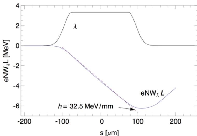
*Dechirper for NGLS: wake of model of NGLS bunch distribution (blue). The dashed, red line gives the linear chirp approximation. The bunch shape  $\lambda$ , with the head to the left, is given in black*
