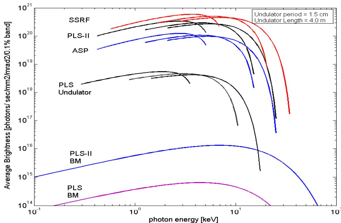
ID radiation brightness from the PLS-II is expected to be  $2 \times 10^{20}$  photons/sec/mm<sup>2</sup>/mrad<sup>2</sup>/0.1%BW (@ 10 keV (1 )) which is about 100 times brighter than the existing PLS.
