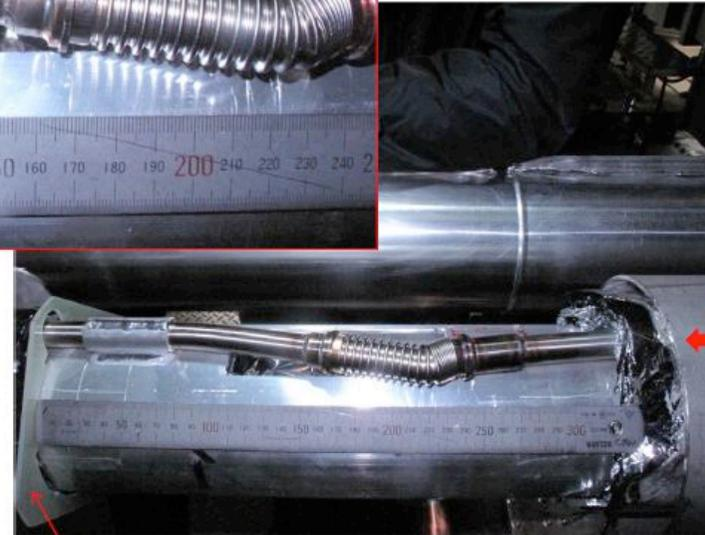
LN2 line spacer must be at upstream of LN2 flow, but it is at downstream.
