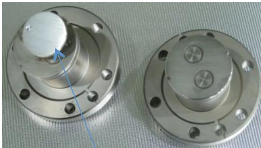
Pickup antenna on BPM electrode
