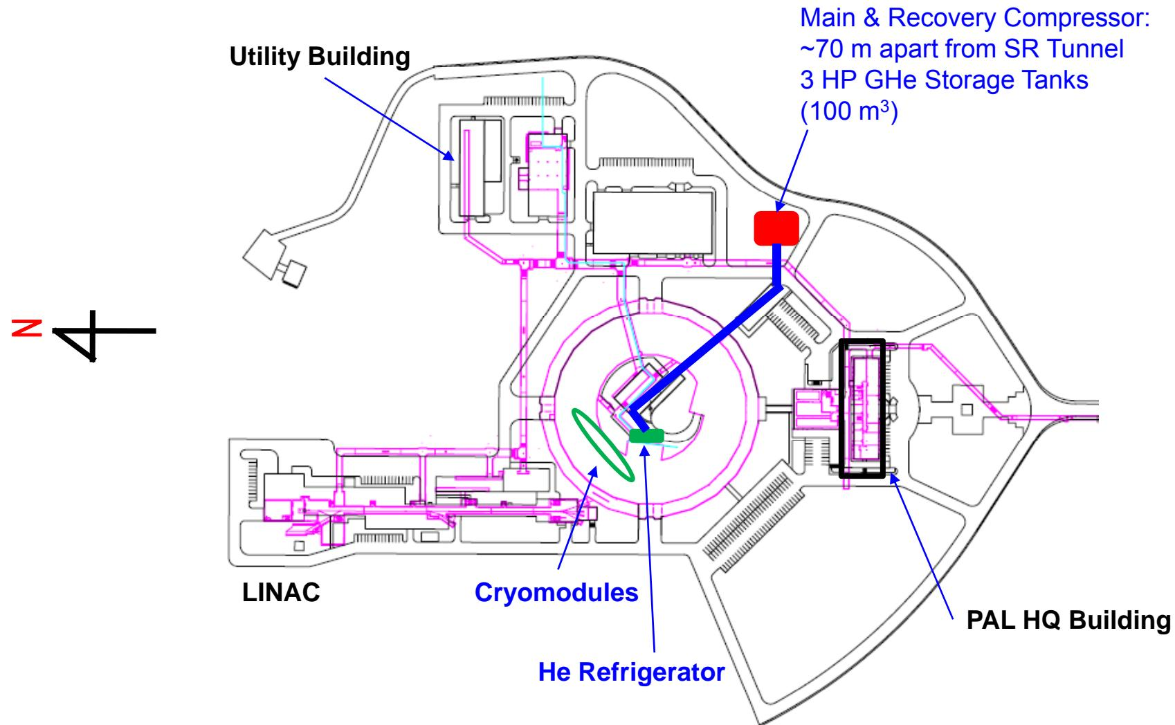
Pink Line: Underground Tunnel for utility like piping, wires
