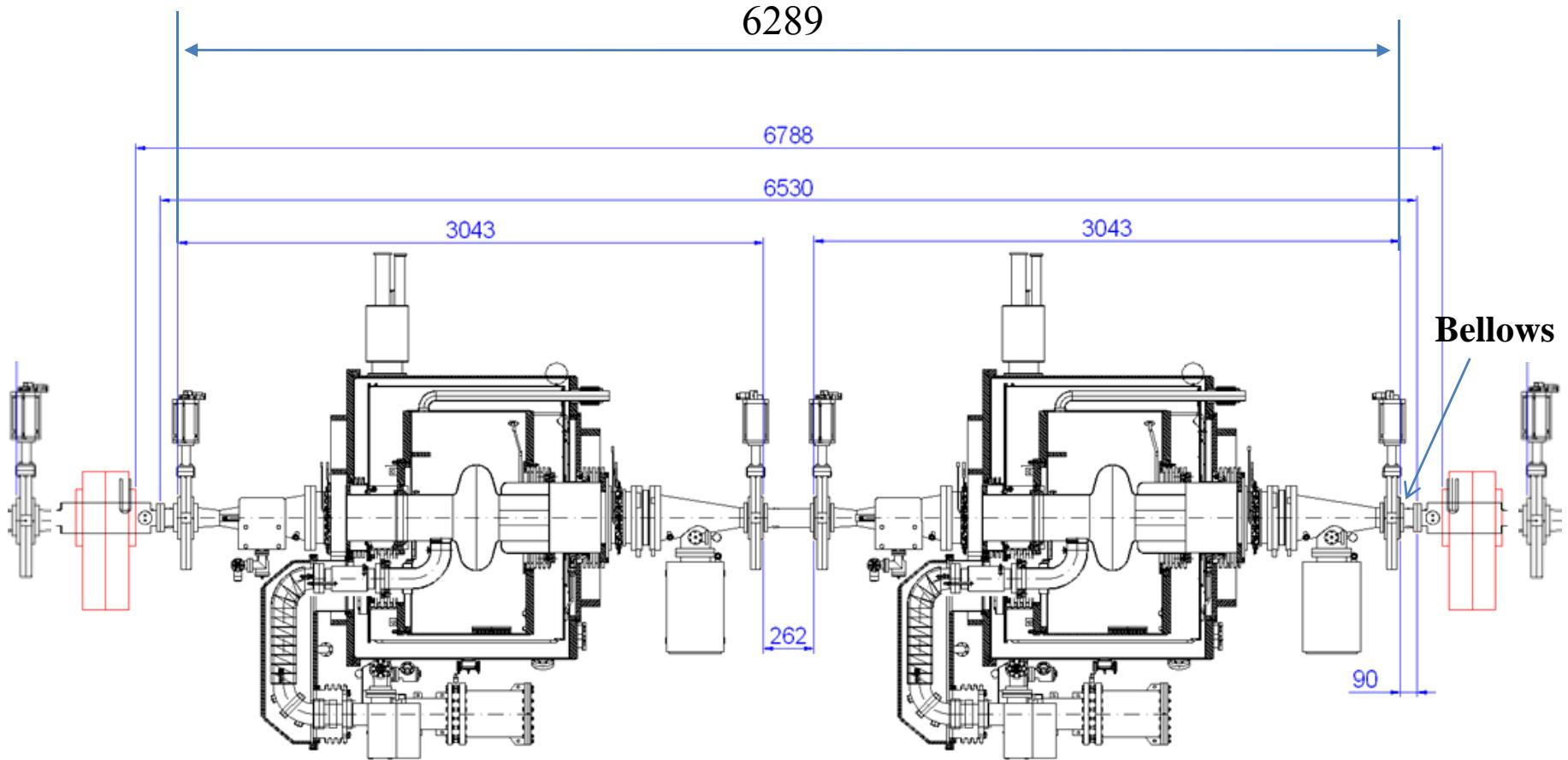
Two CESR-type cryomodules in a long-straight section.
