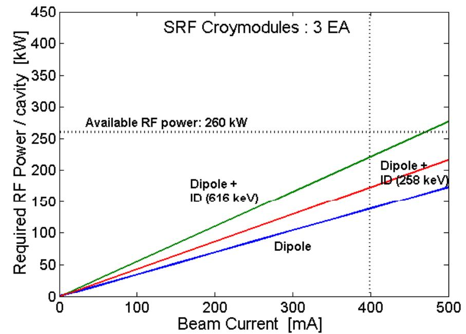
With two cryomodules, 210 kW is required to compensate dipole radiation loss at 400 mA current
