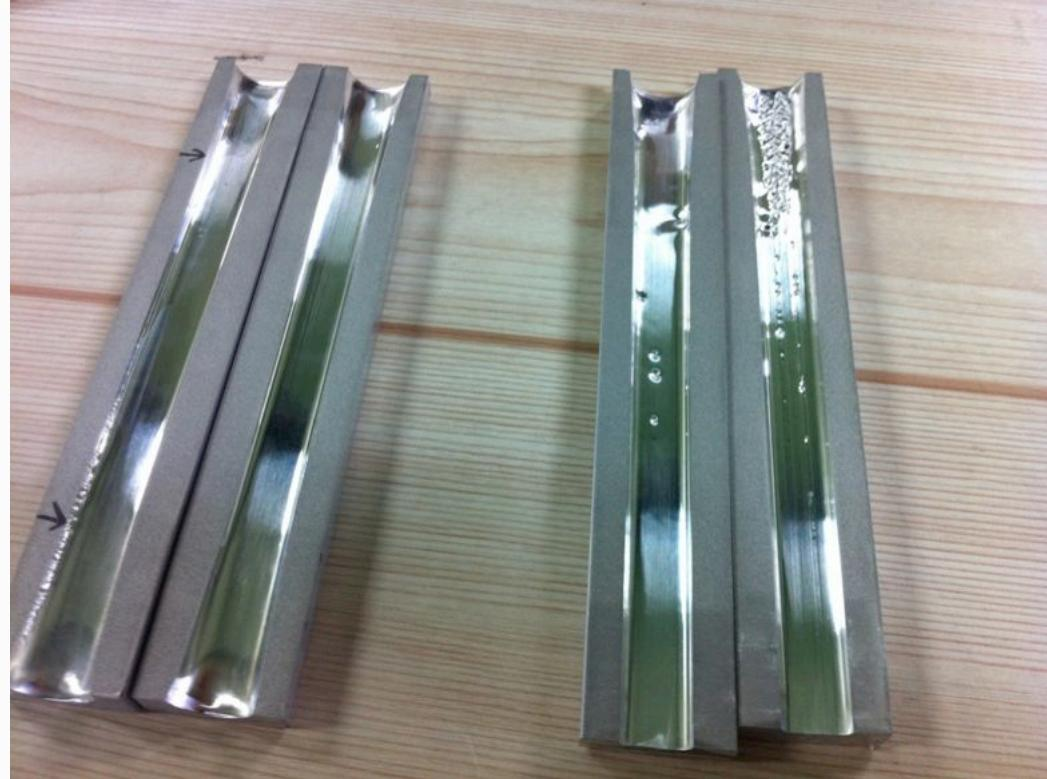
Pits have been found on the polished surface of the test specimens.
