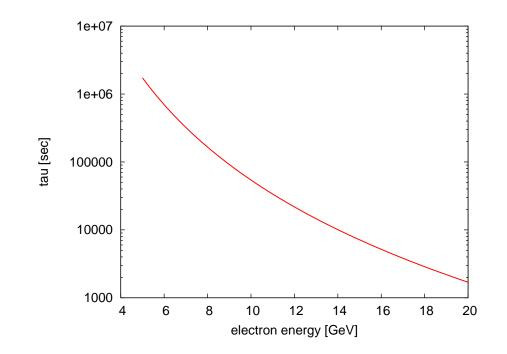
Self-polarization is not viable except at highest energies ⇒ Need a full-energy polarized injector Advantage of a full-energy polarized injector:
