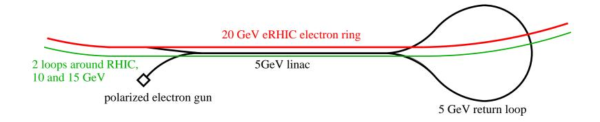
Acceleration up to 10 GeV in one 200 m long RHIC straight, plus two recirculating loops at 15 and 20 GeV around entire RHIC tunnel 3. Highly symmetric rapid-cycling (or rapid-ramping) synchrotron (RCS)
