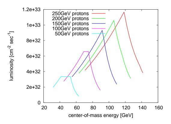
Ring-ring approach provides up to 1.2 · 10<sup>33</sup> cm<sup>-2</sup>sec<sup>-1</sup> luminosity over the required energy range, depending on beam energies
