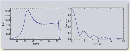
Beam spectrum extends to 2-3 THz, the wavelengths  $100-150~\mu m$ .
