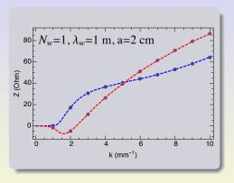
Remarkably, the parallel plate model agrees well with the rectangular cross section impedance with the aspect ratio  $b/a \gtrsim 2-3$ .
