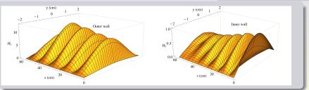
The unit of H is the magnetic field in the straight pipe (the heating from the image currents is  $\approx 1.5 \text{ mW/cm}^2$ ). We estimate the energy deposition on the outer wall of the toroid  $\sim 0.2 \text{ W/cm}^2$ .
