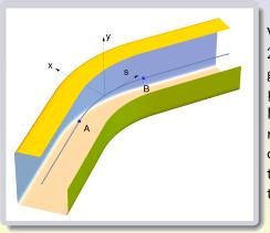
Vacuum chamber: full vertical gap 2h=3.2 cm, and the full horizontal gap 9.6 cm. The beam radiates 113  $\mu J$  energy (113 W); this agrees with M. Dohlus's two-parallel-plates result: 120  $\mu J$ . Also, the wakefields calculated at various distances from the exit of the bend agree between the two codes.
