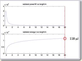
The long tail of the wake is due to the edge radiation of the beam. In the limit  $\gamma \to \infty$  the total radiated energy  $\to \infty$ .
