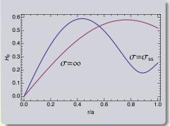
Radial dependence of the magnetic field in  $TM_{01}$  for a perfectly conducting and ss pipe (f=1.9 THz, a=2 cm). The attenuation is actually  $\alpha=0.13$  m<sup>-1</sup>.
