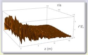
Distribution of  $r|E_r(r,z)|$  for the radiation field in the pipe excited by the beam at 2.4 THz (the total field is the radiation field plus the Coulomb field of the beam).
