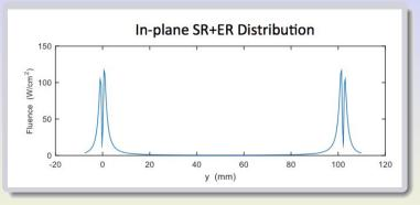
The peaks are due to the edge radiation from the bend.
