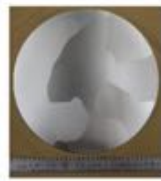
Large Grain (LG)材 φ260mm
