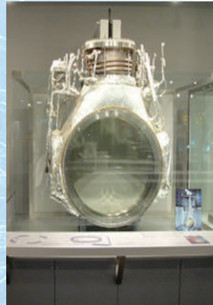
KEK 1m Liquid Hydrogen Bubble Chamber
