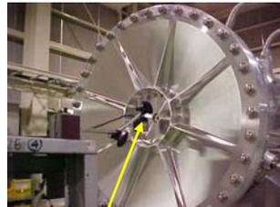
Parabolic disk with 8 ribs
