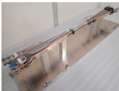
Belle II Beam Pipe
