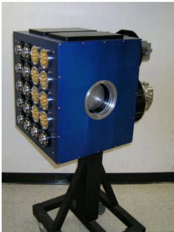
64-pixel heterodyne imaging spectrometer (SuperCam) [1]
