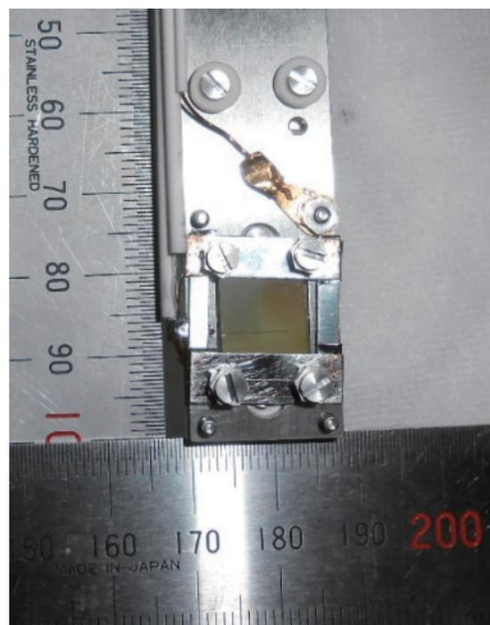
**Fig. 6:** BaTiO<sub>3</sub> substrate mounted on a sample holder for the XMCD measurement, by which up to  $\pm 1$  kV is applied between the surface and the bottom of the substrate.
