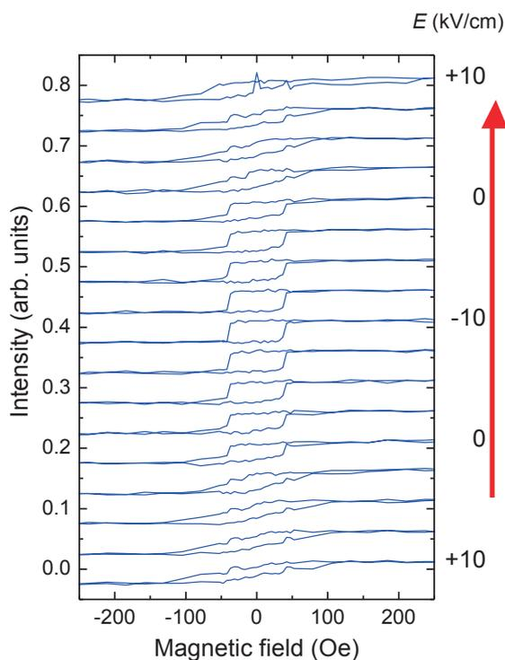
**Fig. 7:** Applied voltage dependence of the magnetization curve for FeCo/BaTiO<sub>3</sub>(001) taken by using Fe L-edge XMCD at the grazing incidence configuration at room temperature.
