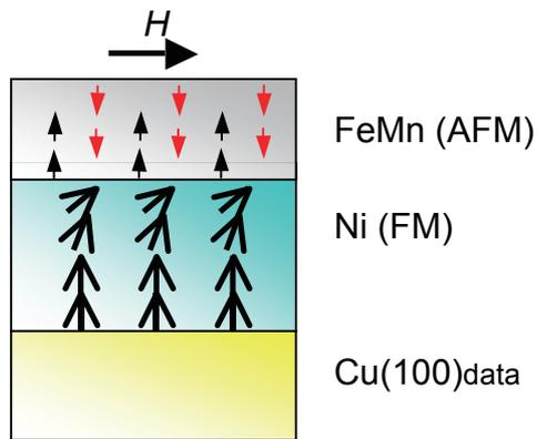
**Fig. 5:** Schematic illustration of magnetic structure of FeMn/Ni/Cu(100) under a weak in-plane magnetic field,  $H$ . The Ni magnetic moment gradually rotates from the perpendicular to in-plane directions as approaching the interface to AFM FeMn.
