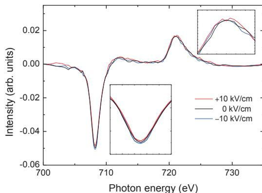
**Fig. 8:** Fe L-edge XMCD spectra taken by applying different voltages to FeCo/BaTiO<sub>3</sub>(001).
