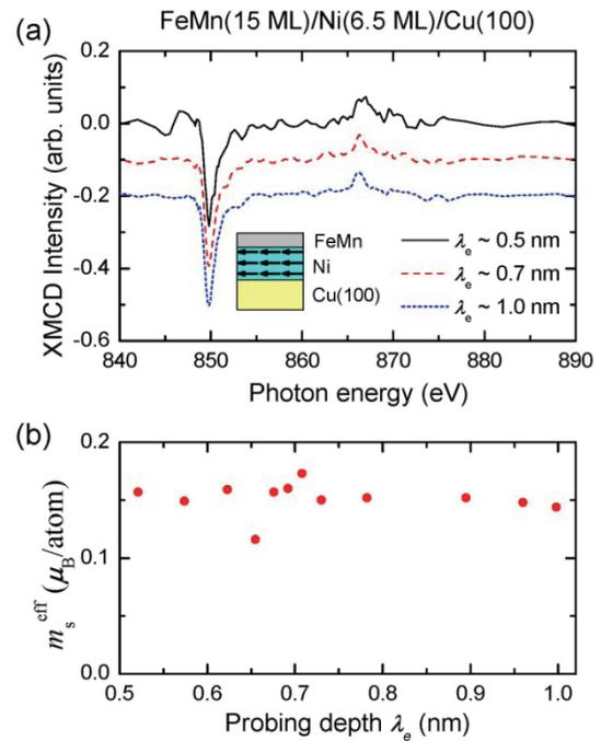
**Fig. 2:** Probing depth ( $\lambda_e$ ) dependence of (a) grazing-incidence Ni L-edge XMCD spectrum for FeMn(15 ML)/Ni(6.5 ML)/Cu(100) and (b) averaged effective spin magnetic moment  $m_s^{\text{eff}}$  estimated by applying the sum rules to each spectrum.
