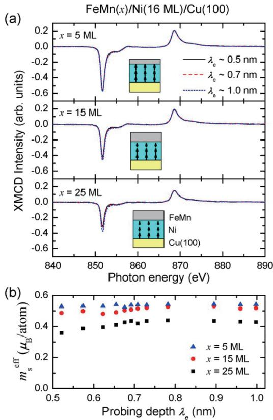
**Fig. 1:** Probing depth ( $\lambda_e$ ) dependence of (a) normal-incidence Ni L-edge XMCD spectrum for FeMn(x)/Ni(16 ML)/Cu(100) and (b) averaged effective spin magnetic moment  $m_s^{\text{eff}}$  estimated by applying the sum rules to each spectrum.
