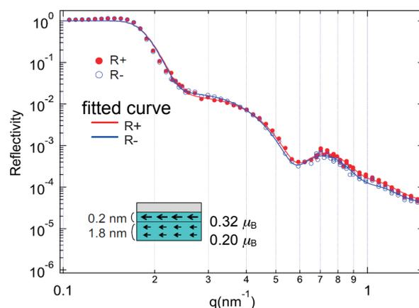
**Fig. 4:** Observed and fitted PNR curves, R+ and R-, for Cu(74 ML)/FeMn(21 ML)/Ni(11 ML)/Cu(100) film measured at a magnetic field of 1 kOe. The magnetic field is parallel to the quantization axis of the neutron and is perpendicular to the surface normal direction. The magnetic structure model used in the fitting procedure is shown in the inset.
