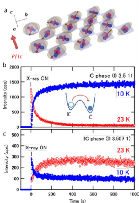
**Fig. 3:** (a) Magnetic structure of Mn spins in the *bc*-cycloidal incommensurate phase of  $\text{Gd}_{0.5}\text{Tb}_{0.5}\text{MnO}_3$ . X-ray irradiation time dependence of super-lattice diffraction intensities for (b) the commensurate (C) (0, 3.5, 1) reflections and for (c) the incommensurate (IC) (0 3.507 1) reflections.
