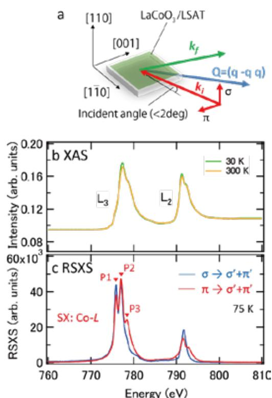
**Fig. 1:** Schematic drawing of the grazing-incident resonant soft X-ray scattering (GI-RXS). The diffracted soft X-rays ( $k_f$ ) were observed with the incident soft X-rays ( $k_i$ ) in the grazing angle condition. The scattering plane was tuned nearly parallel to the sample surface. XAS and RSXS spectra at the Co  $L_{2,3}$ -edge of  $\text{LaCoO}_3/\text{LSAT}(110)$  thin film.
