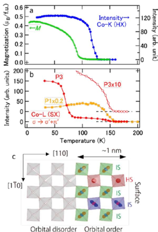
**Fig. 2:** Temperature dependence of (a) magnetization (M) and intensity of super-lattice peaks at  $(2 + q, 2 - q, q)$  with  $q = 1/4$  measured by hard X-ray diffraction (HX), (b) intensities of super-lattice peaks at  $(q, -q, q)$  for P1 and P3 of GIRSXS (SX). (c) Schematic picture of the surface freezing and bulk melting of orbital order.
