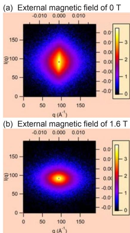
**Fig. 1:** SANS images of a nanocrystalline Nd-Fe-B magnet in the initial magnetization process.
