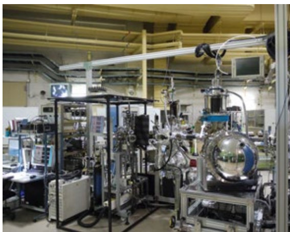
Fig. 2: Photo of the developed in-situ ARPES – laser MBE system installed at the MUSASHI beamline.
