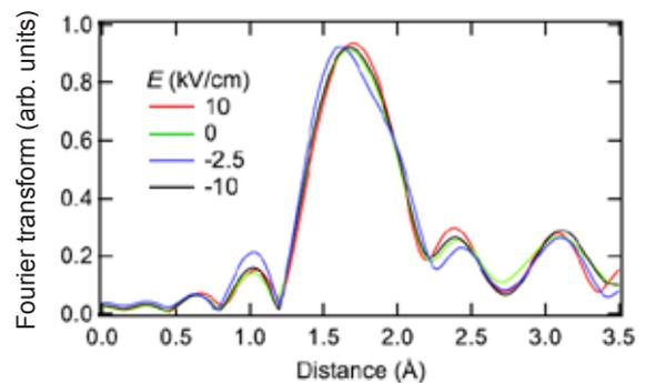
**Fig. 7:** Fourier transforms of the Fe K-edge EXAFS function  $k^2(k)$  of 8 nm Fe film on the BTO substrate.
