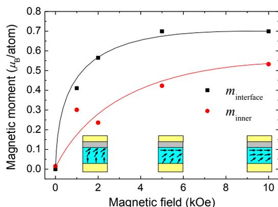
**Fig. 3:** In-plane component of the magnetic moment in the interface and inner region of the Ni film, estimated by fitting the PNR curves, as a function of applied magnetic field,  $H$ . The lines are guides for the eye. The expected magnetic structure is schematically illustrated.
