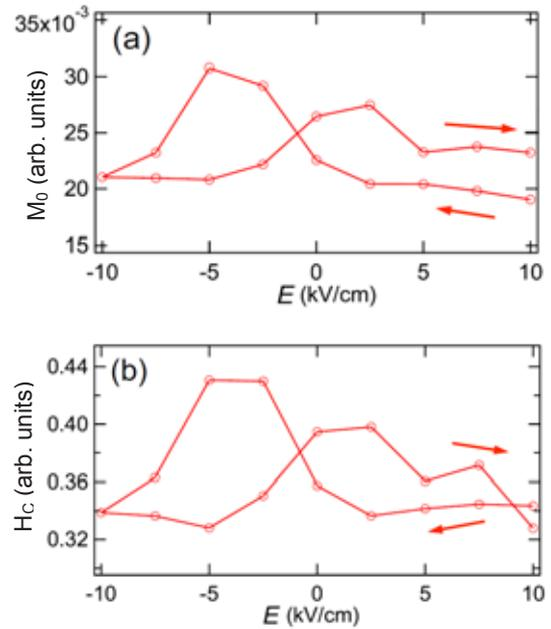
**Fig. 5:** Electric field dependence of the residual magnetization,  $M_0$  (a), and the coercive field,  $H_c$  (b). The electric field is changed from 10 kV/cm, as indicated by the arrows.
