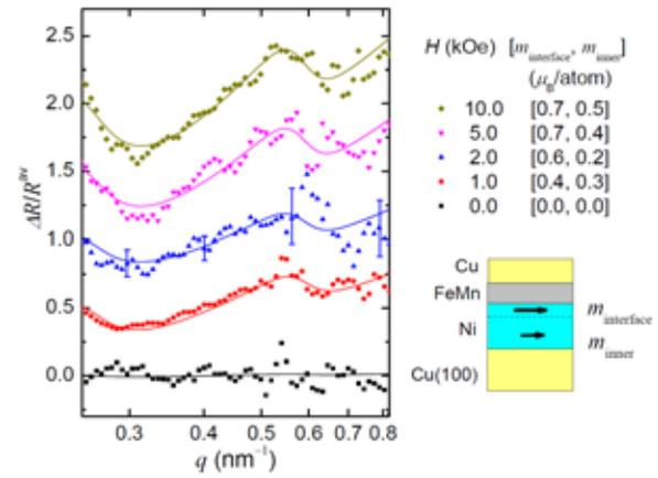
**Fig. 2:** Difference in the PNR curves,  $\Delta R = R^+ - R^-$ , divided by the average of them,  $R_{av} = (R^+ + R^-)/2$ , for Cu/FeMn/Ni/Cu(100) measured at different magnetic fields,  $H$ . The data for different  $H$  are vertically shifted. The lines are the simulated curves using the in-plane magnetic moments in the interface and inner regions of the Ni film,  $m_{interface}$  and  $m_{inner}$ , respectively, indicated in the figure.
