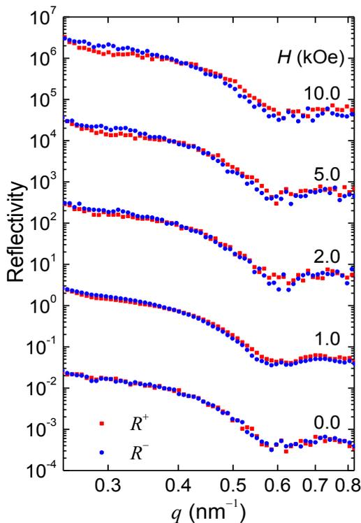
**Fig. 1:** PNR curves,  $R^+$  and  $R^-$ , for Cu/FeMn/Ni/Cu(100) measured at different magnetic fields,  $H$ . The data for different  $H$  are vertically shifted.
