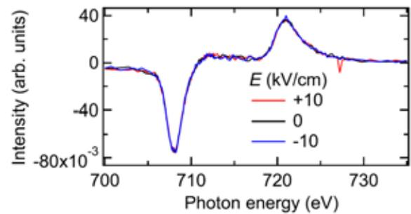
**Fig. 6:** XMCD spectra of 8 nm Fe film on the BTO substrate measured at the electric field of +10, 0 and -10 kV/cm.
