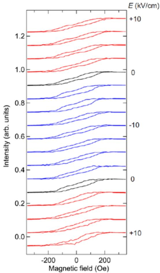
**Fig. 4:** XMCD-hysteresis curves measured at Fe  $L_3$  absorption edge of 8 nm Fe thin film on the BTO substrate at different electric fields,  $E$ .
