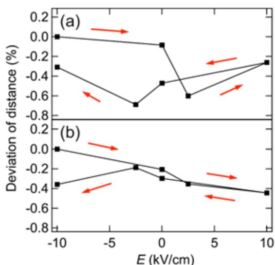
**Fig. 8:** Deviation of the in-plane bond distances for Fe-O (a) and Fe-Fe (b), as a function of the electric field,  $E$ . The electric field is changed from  $E = -10$  kV/cm, as indicated by the arrows.
