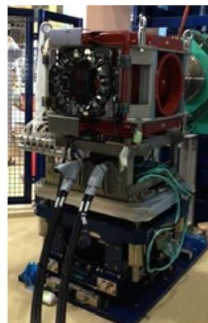
**Fig. 6:** New spectrometer for the muon spin relaxation measurement installed at the S1 experimental area.
