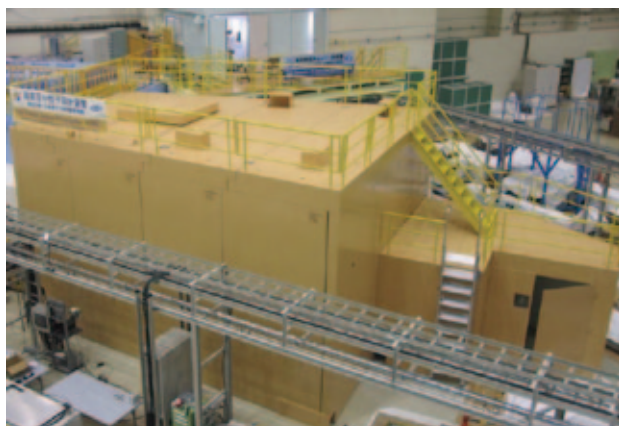
Fig. 9 New high-pressure neutron beamline PLANET, in which the six-axis large volume press will be installed in FY 2011.
