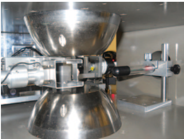
Fig. 6: Experimental setup for polarized neutron reflectivity at BL-17 in J-PARC.
