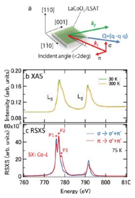
**Fig. 1:** Schematic drawing of the grazing-incident resonant soft X-ray scattering (GI-RSXS). The diffracted soft X-rays ( $k_i$ ) were observed with the incident soft X-rays ( $k_i$ ) in the grazing angle condition. The scattering plane was tuned nearly parallel to the sample surface. XAS and RSXS spectra at the Co  $L_{2,3}$ -edge of LaCoO<sub>3</sub>/LSAT(110) thin film.
