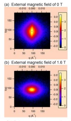
**Fig. 1:** SANS images of a nanocrystalline Nd-Fe-B magnet in the initial magnetization process.
