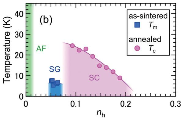
**Fig. 6:** Magnetic ( $T_m$ ) and superconducting (SC) transition temperatures ( $T_c$ ) in as-sintered and oxidation annealed  $\text{La}_{1-x/2}\text{Eu}_{1-x/2}\text{Sr}_x\text{CuO}_4$  as a function of the hole density ( $n_h$ ). Green, blue, and pink areas represent the antiferromagnetic ordered (AF), spin-glass (SG), and SC states, respectively. Solid lines are guides to the eyes.
