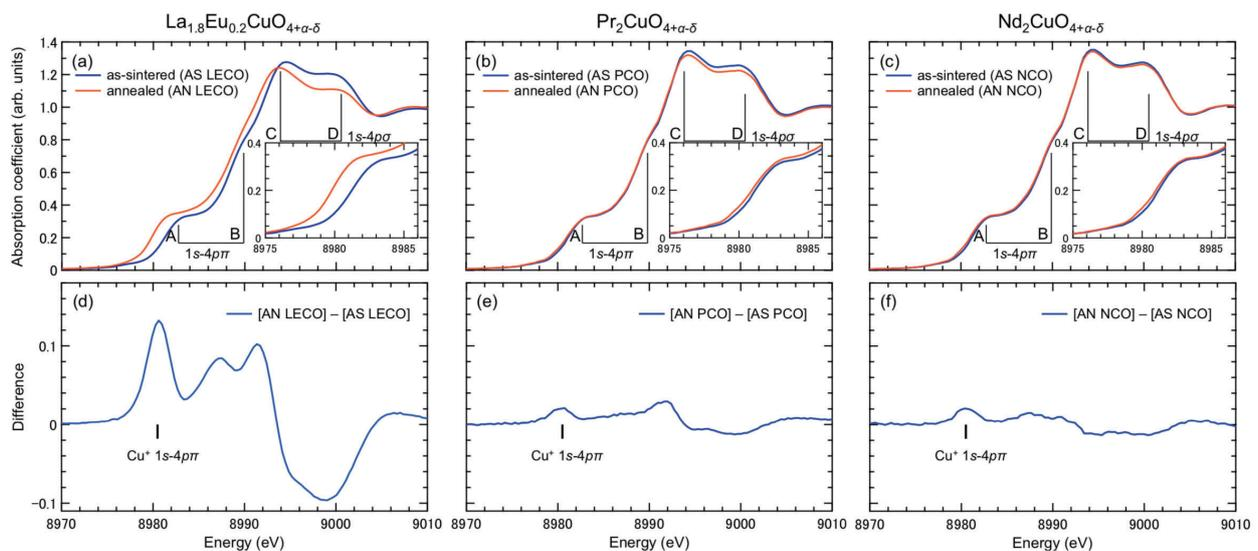
**Fig. 3:** (a) XANES spectra for as-sintered and annealed (a)  $\text{La}_{1.8}\text{La}_{0.2}\text{CuO}_4$ , (b)  $\text{Pr}_2\text{CuO}_4$  and (c)  $\text{Nd}_2\text{CuO}_4$ . Differential spectra between annealed and as-sintered (d)  $\text{La}_{1.8}\text{La}_{0.2}\text{CuO}_4$ , (e)  $\text{Pr}_2\text{CuO}_4$  and (f)  $\text{Nd}_2\text{CuO}_4$ .
