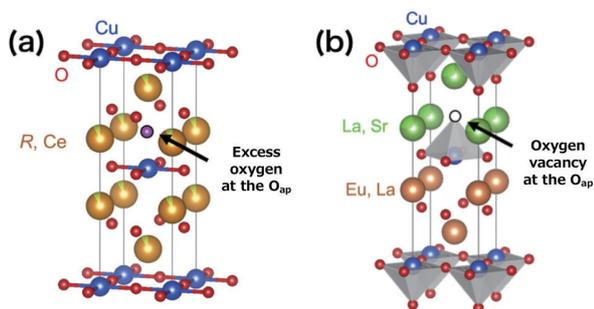
**Fig. 1:** Crystal structure of  $\text{R}_2\text{CuO}_{4+\delta}$ . ( $\text{R}$ : rare earth) with (a)  $T$ - and (b)  $T^*$ -type cuprates.  $T$ ( $T^*$ )-type cuprate has flat  $\text{CuO}_2$  planes ( $\text{CuO}_5$  pyramid) with four (five) coordination for Cu ions. In the AS  $T$ ( $T^*$ )-type cuprate, excess oxygen (oxygen vacancy) is considered to exist at an apical oxygen site.
