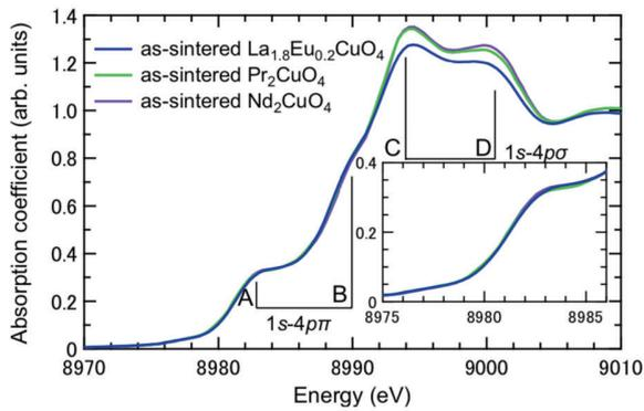
**Fig. 2:** XANES spectra for as-sintered powder samples of  $\text{La}_{1.8}\text{Eu}_{0.2}\text{CuO}_4$ ,  $\text{Nd}_2\text{CuO}_4$  and  $\text{Pr}_2\text{CuO}_4$ . The inset is the enlarged spectra in the range from 8975 eV to 8986 eV.
