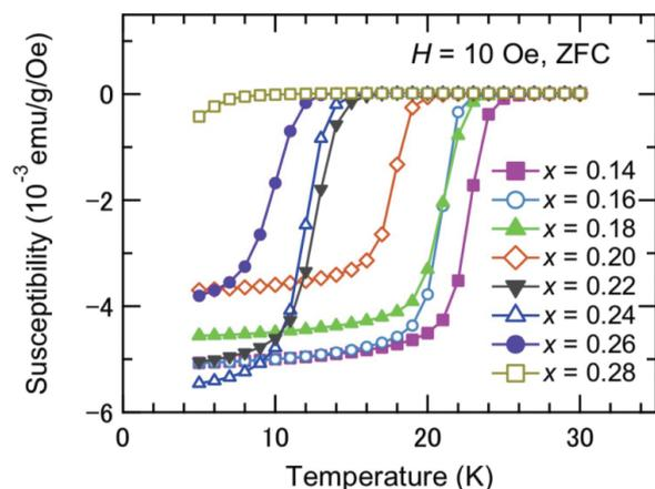
**Fig. 4:** Temperature dependence of magnetic susceptibility measured after zero-field-cooling process for the oxidation annealed *T*\*-La<sub>1-x/2</sub>Eu<sub>1-x/2</sub>Sr<sub>x</sub>CuO<sub>4</sub>.
