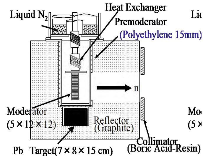
6 times higher intensity than the traditional one, and twice higher than a decoupled methane moderator.
