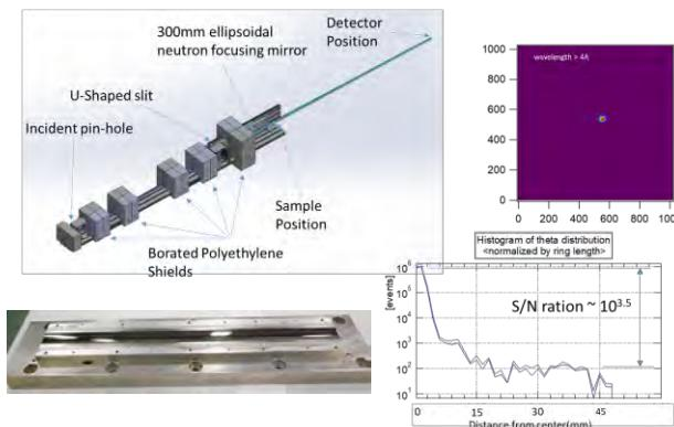
A 300mm ellipsoidal neutron focusing mirror for focusing SANS beamline at RANS
