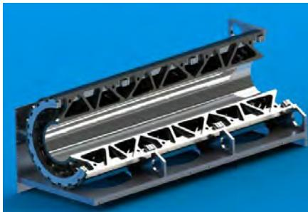
A fully-revolved 900mm ellipsoidal neutron focusing mirror for J-PARC BL-06 VIN ROSE
