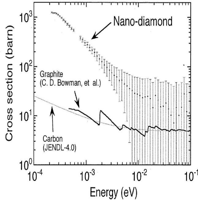
Fig. 8 Total cross sections of nano-diamond. Cross section of carbon (JENDL-4.0, [21]) and graphite (C. D. Bowman et al., [22]) are shown for comparison
