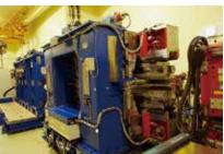
The development of insertion device technologies such as undulators has made it possible to obtain high-brightness, polarization-controlled light (photo: undulator at BL-2).
