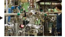
The processed light is irradiated onto the sample and data are acquired (photo: in situ high-resolution angle-resolved photoemission spectrometer installed at BL-2).
