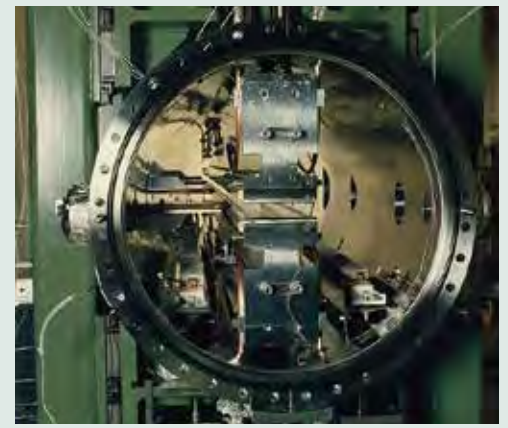
The first in-vacuum undulator (AR-NE3)
