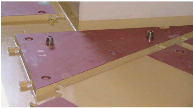
Fig. 2. Alignment plate with pivots used to position and align beamline components.
