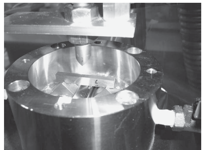
Fig. 8. The picture of the bending test, in which a specimen with the tilted interface was tested.
