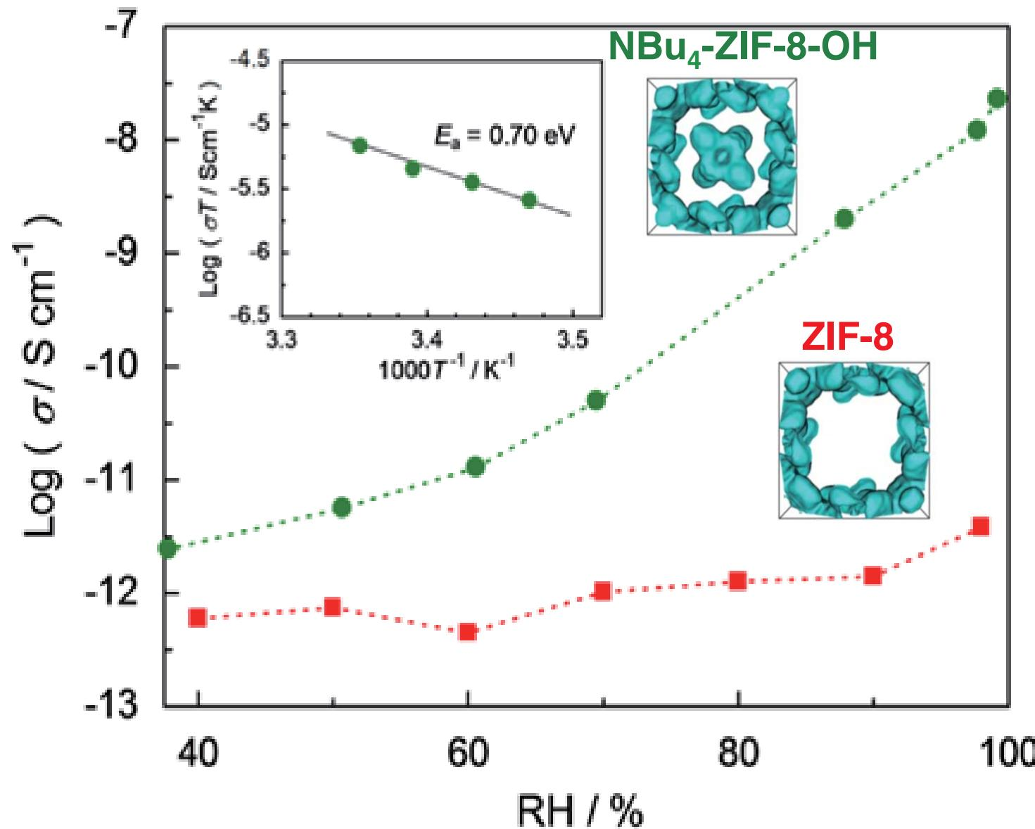
Ionic conductivity of  $\text{NBu}_4\text{-ZIF-8}$  exhibits 4 orders of magnitude higher ionic conductivity than that of the blank ZIF-8 inclusion.
