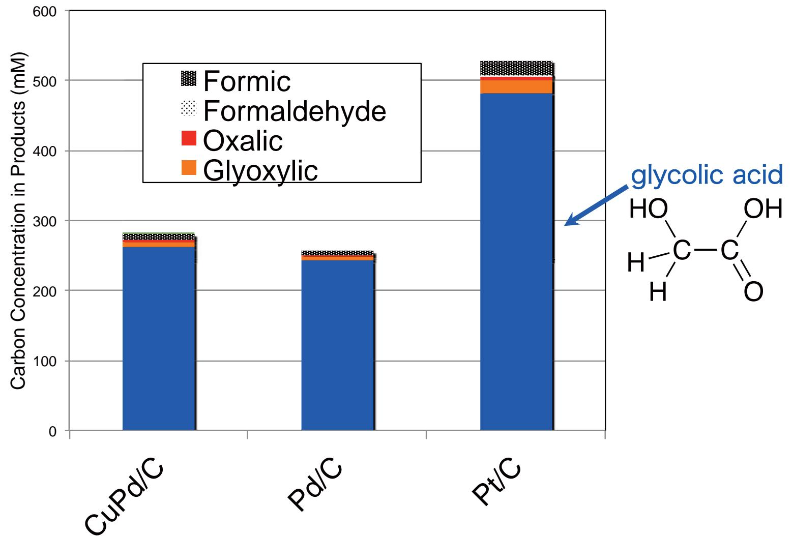
EG can be oxidized to **glycolic acid** (**4e-oxidation**) on Pt-group catalysts.
