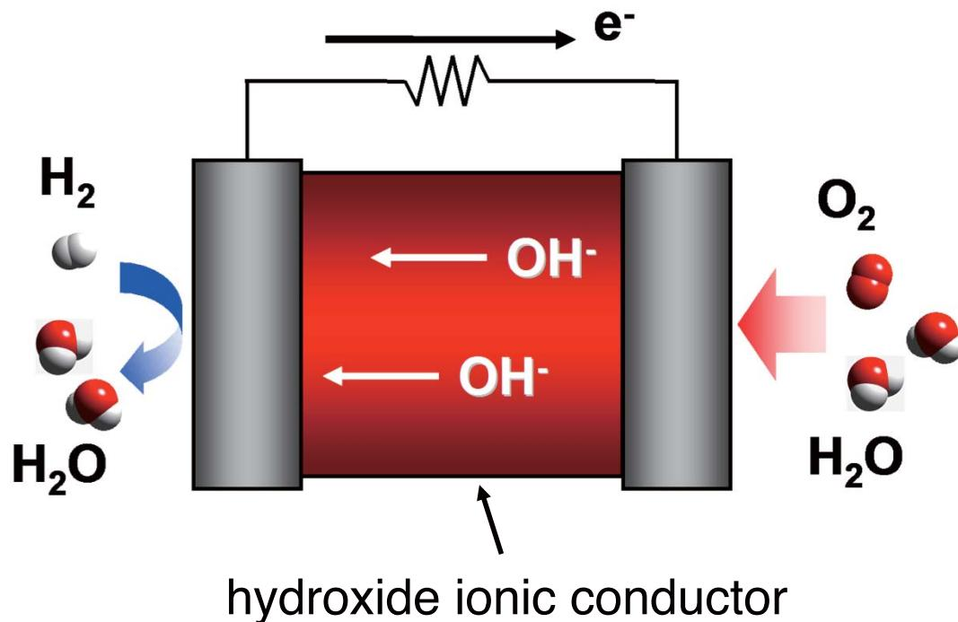
Development of novel hydroxide ionic conductor is indispensable for practical use of alkaline fuel cells.
