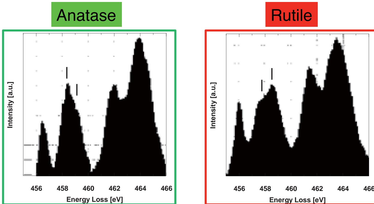
\*measured using JSM-ARM200F installed in Next-Generation Fuel Cell Research Center (NEXT-FC), Kyushu University
