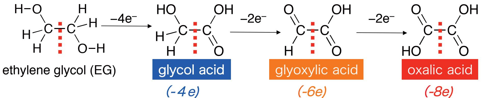
EG oxidation to oxalic acid without C-C cleavage
