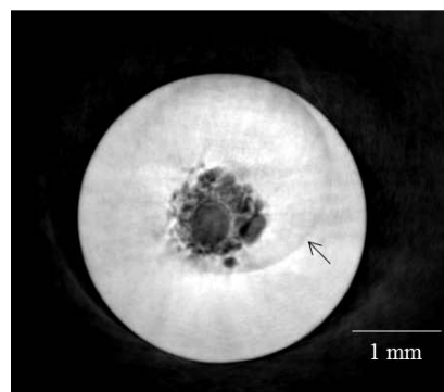
Figure 4 Tomogram slice of the reconstructed \delta(x, y, z) of the PE sphere.
