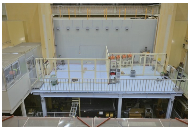
Figure 1 View of the test beam area (beam stage) for users in AR South building. The left area inside the fence is for users, and the right for beam extraction components such as quadrupole magnets and beam shutter.
