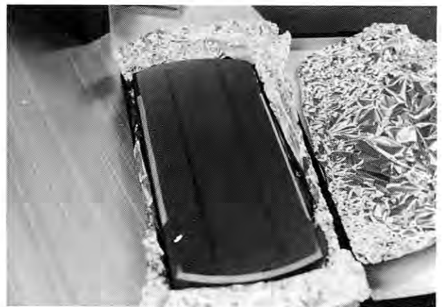
Fig. 3.2.4 Pt-coated flat SiC mirror having been used on the grasshopper line. It has a size of 40 \times 17 \times 4 \text{ cm}^3 .
