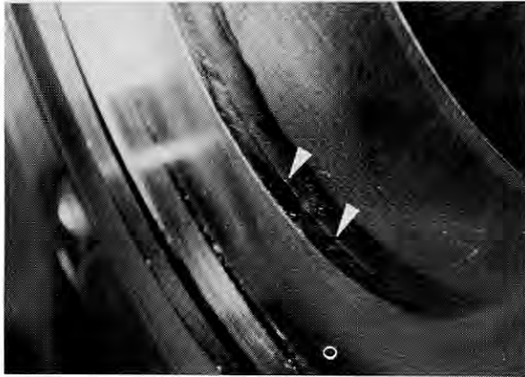
Fig. 2.3.13 Photograph of the tuner flange. The oil-like liquid is seen at three points.
