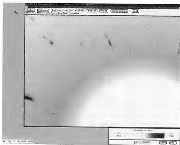
Fig.17 The Laue pattern of 3.5\ \mu\text{m} area of a thin section of a meteorite taken for 60min. with the ring current from 176 to 175mA.
