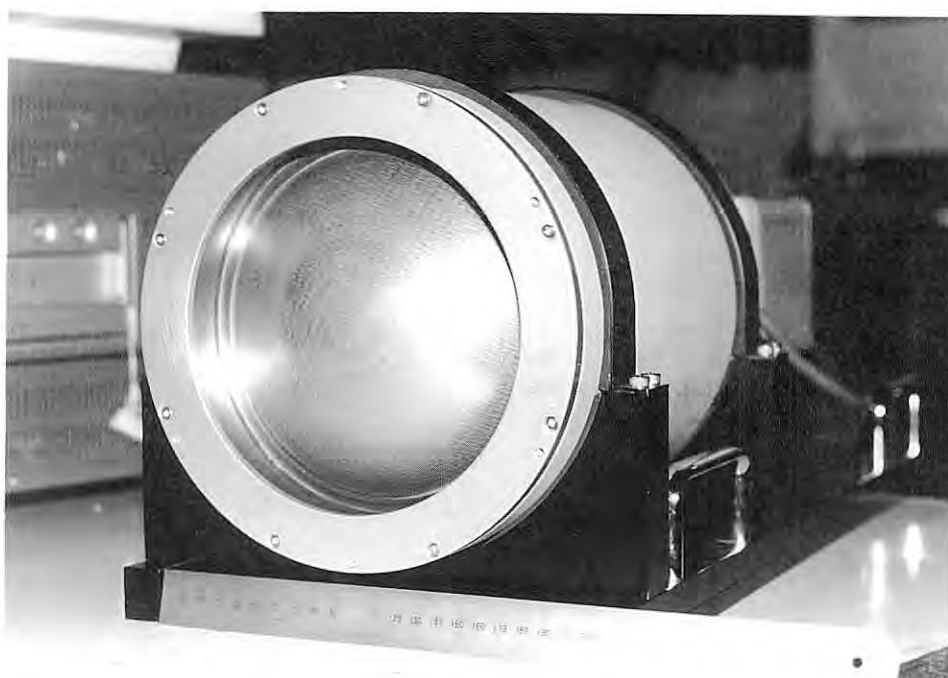
Fig. 14 Front view of the X-ray TV detector, which utilizes a beryllium-windowed (1 mm thick) X-ray image intensifier.
