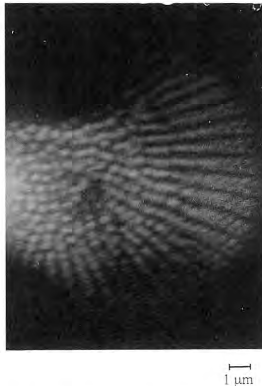
Fig. 6 Magnified image of dry diatoms. The X-ray wavelength was 2.37 nm. The magnification of the X-ray optical system was about 1020. The exposure time was about 2 min. A scale mark is 1 \mu m.
