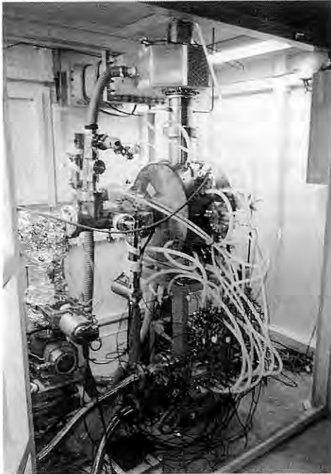
Fig. 23 High-power test cavity mounted on a test bench.
