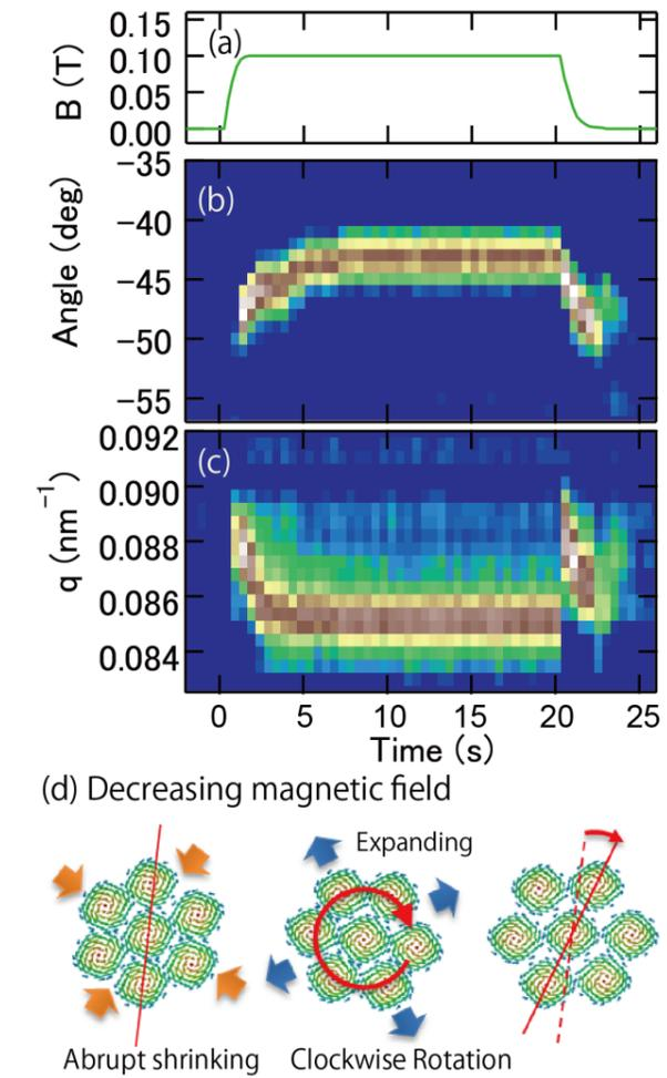
**Figure 3:** Temporal change of applied magnetic field (a), azimuthal angle  $\phi$  (b), and magnitude of  $q$  vector ( $q = |q|$ ) (c) of magnetic scattering from helical and SkX magnetic structures. (d) Schematic pictures of transient variation in magnetic structure from the SkX to helical magnetic structure with decreasing magnetic field.
