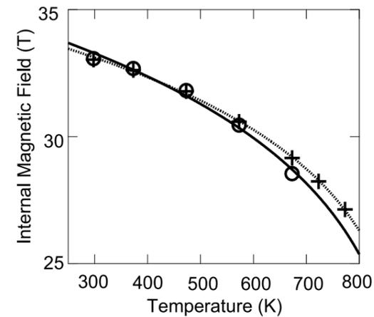
**Figure 2** Temperature dependence of  $B_{hf}$  taken for  $^{56}\text{Fe}/^{57}\text{Fe}/\text{MgO}(001)$  (O) and  $^{56}\text{Fe}/^{57}\text{Fe}/^{56}\text{Fe}/\text{MgO}(001)$  (+). Solid and dotted curves are fits with a common  $T_c$  value to the data of the former and latter samples, respectively.
