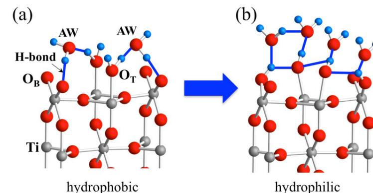
**Figure 2:** Structural models of the (a) hydrophobic and (b) hydrophilic surfaces. Hydrogen bonds are represented by light-blue lines.
