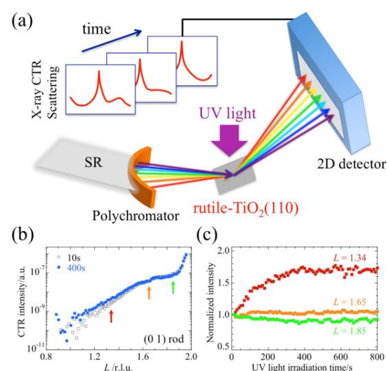
**Figure 1:** (a) A schematic illustration of the time-resolved CTR measurement in wavelength-dispersive mode during UV-light irradiation on the rutile-TiO<sub>2</sub>(110) surface. (b) Scattering intensity profiles of the (01L) rod measured at the photoirradiation ( $\lambda = 365$  nm, 87 mW/cm<sup>2</sup>) time of 10 s and 400 s. (c) Time evolutions of the normalized intensity at selected points (indicated by arrows in (a)) of the (01L) rod.
