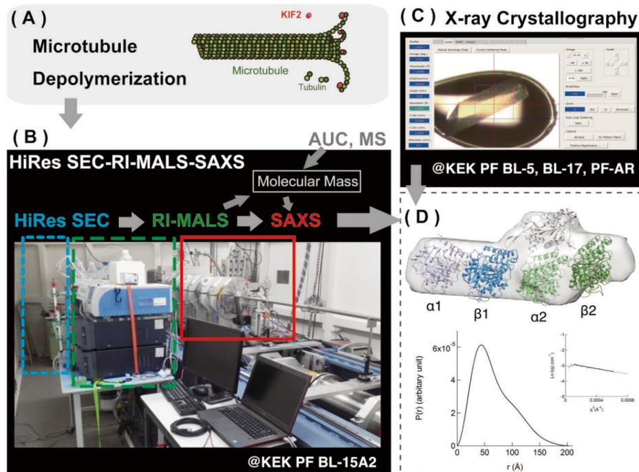
**Figure 1:** Combination of multiple X-ray based approaches at PF. (A) Microtubules (MTs) are dynamic polymer cytoskeletons composed of  $\alpha$ - $\beta$ -tubulin dimers. KIF2 depolymerizes MTs. (B) HiRes SEC-SAXS system at BL-15A2. (C) X-ray crystallography beamline. (D) SAXS model of KIF2-tubulin complex.
