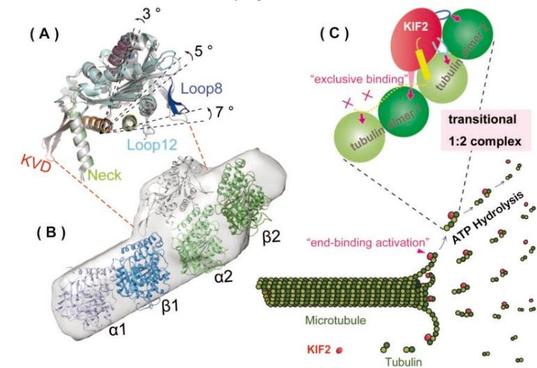
**Figure 2:** Mechanism of microtubule depolymerization. (A) Transitional conformation of KIF2 structure revealed by X-ray crystallography. (B) Transitional conformation of KIF2-tubulin 1:2 complex revealed by SAXS analysis. (C) Model of the efficient mechanism of microtubule depolymerization via transitional KIF2-tubulin complex.
