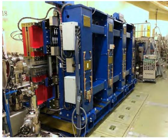
**Figure 5:** New APPLE-II type undulator installed for BL-19.
