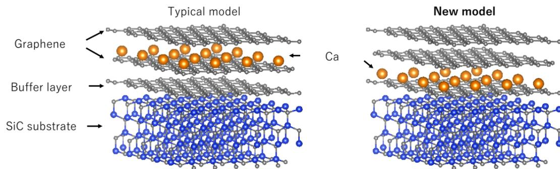
**Figure 1:** Comparison of the structure models of Ca-intercalated bilayer graphene on SiC(0001) between a typical conventional model (left) and the new model (right) determined by this study.
