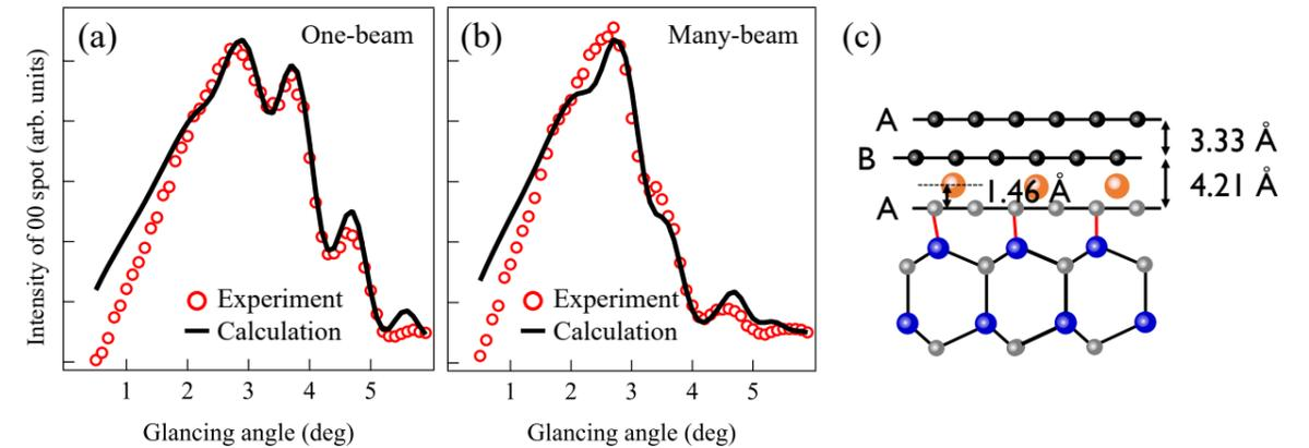
**Figure 2:** TRHEPD rocking curves under the (a) one-beam condition with calculated curves and (b) the many-beam condition with the calculated curves for Ca-intercalated graphene on SiC(0001). (c) Schematic view of the structure determined for Ca-intercalated graphene on SiC(0001).
