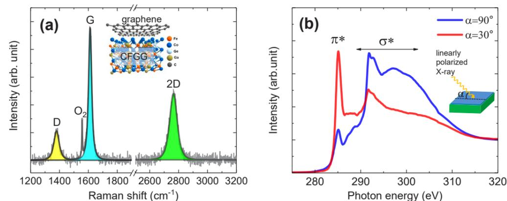
**Figure 1:** (a) Raman spectrum of SLG/CFGG heterostructure. (b) C  $K$ -edge XAS spectra measured at the incident angles of  $\alpha = 30^\circ$  (red solid line) and  $\alpha = 90^\circ$  (blue solid line). The sharp peak at  $1557 \text{ cm}^{-1}$  of (a) is attributed to  $\text{O}_2$  in ambient air. The inset of (a) is a sketch of the SLG/CFGG heterostructure.
