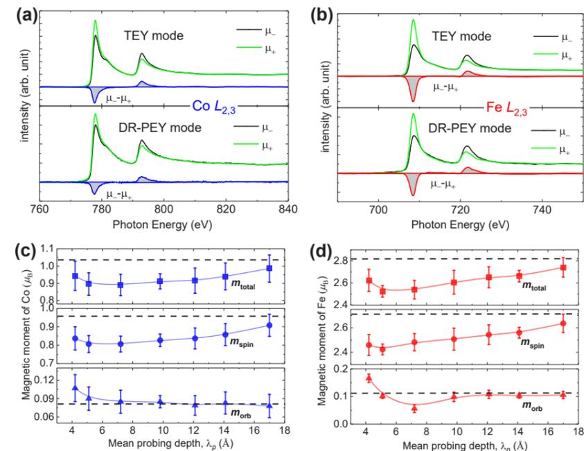
**Figure 2:** (a, b) Comparison of XAS and XMCD spectra of SLG/CFGG heterostructure at Co and Fe  $L_{2,3}$ -edges obtained in TEY and DR-PEY modes. (c, d) Plots for orbital, spin and total magnetic moment of Co, and Fe vs. mean probing depth ( $\lambda_p$ ). The DR-PEY spectra in (a) and (b) are at  $\lambda_p \sim 4 \text{ \AA}$ . The dashed lines in (c) and (d) indicate the magnetic moments evaluated from the TEY XMCD spectra.
