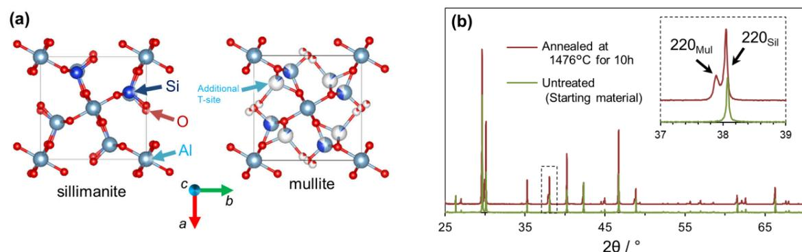
**Figure 1:** (a) Crystal structure of sillimanite and that of mullite (averaged structure). (b) XRD patterns of untreated sillimanite (starting material) and sample annealed at  $1476^\circ\text{C}$  for 10 h in air. The wavelength of the X-ray beam is  $1.747 \text{ \AA}$ .
