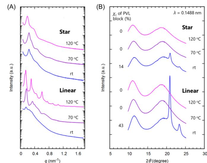
**Figure 2:** Results of simultaneous (A) SAXS and (B) WAXD of *star*- and *linear*-ABCs at various temperatures.
