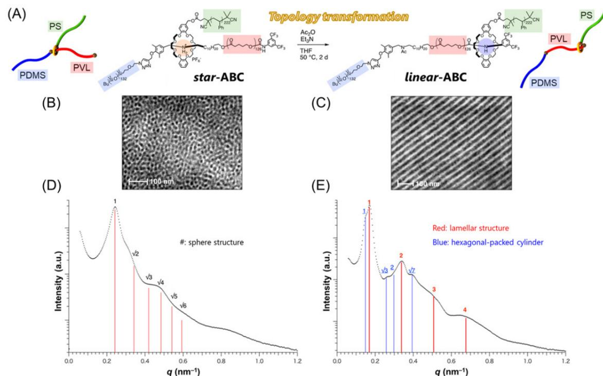
**Figure 1:** (A) A rotaxane-linked ABC *star*-BCP designed to undergo a change in its microphase-separated structure. (B) Bright-field STEM images of *star-ABC* and (C) *linear-ABC*. (D) SAXS profiles of *star-ABC* and (E) *linear-ABC*.
